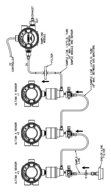
Figure 2-1. Three Ultima X Monitors & a Sampling Module
