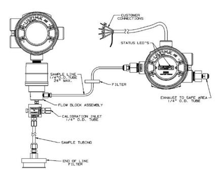
Figure 1-1. Sampling Module Installation with Ultima X Oxygen, Toxic, and Catalytic Combustible Sensors
